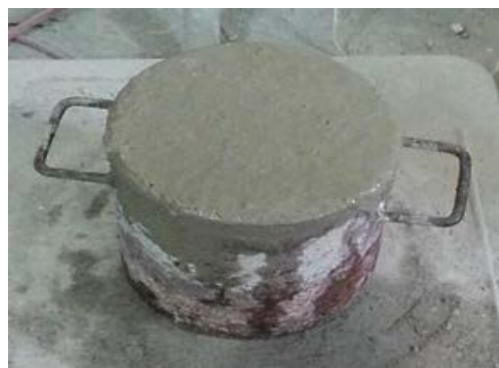
Fig. 3. Determination of bulk specific gravity of concrete mixture
