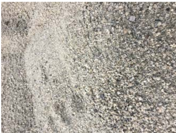
Fig. 2. Granulated blast furnace slag of Tuyen Quang iron steel factory
